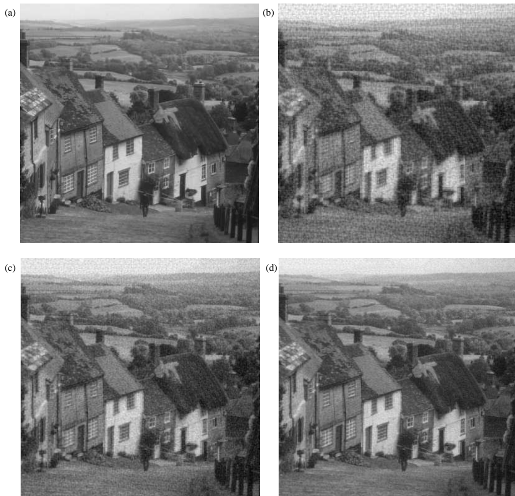
Figure 4.37: Results of the 'goldhill' image at various bitrates (part of training set) using the DCT-based block quantiser: (a) original 8-bit image; (b) 0.25 bits/pixel (PSNR=25.91 dB); (c) 0.5 bits/pixel (PSNR=27.78 dB); (d) 1.0 bits/pixel (PSNR=30.21 dB)
