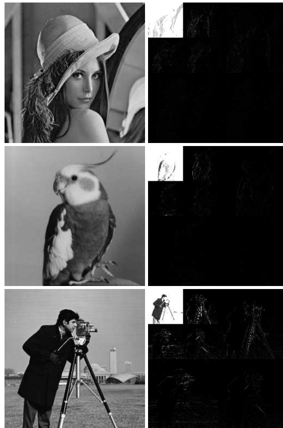
Figure 4.14: Discrete wavelet transform of greyscale test images: ‘lena’, ‘bird’, ‘camera-man’ (using 9/7-tap biorthogonal wavelet filters)
