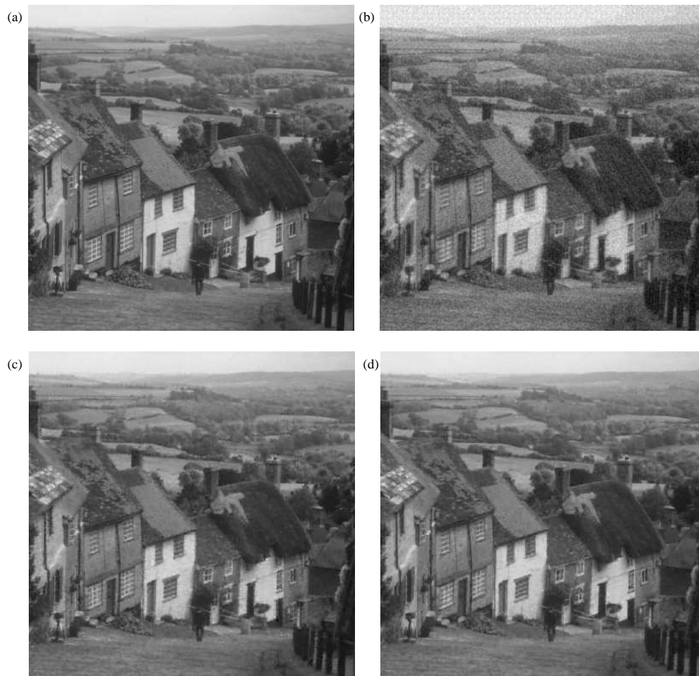
Figure 4.42: Results of the ‘goldhill’ image (part of training set) using the GMM-based block quantiser with varying number of clusters at 0.5 bits/pixel: (a) original 8-bit image; (b) 1 cluster (PSNR=28.08 dB); (c) 4 clusters (PSNR=29.96 dB); (d) 16 clusters (PSNR=30.53 dB)
