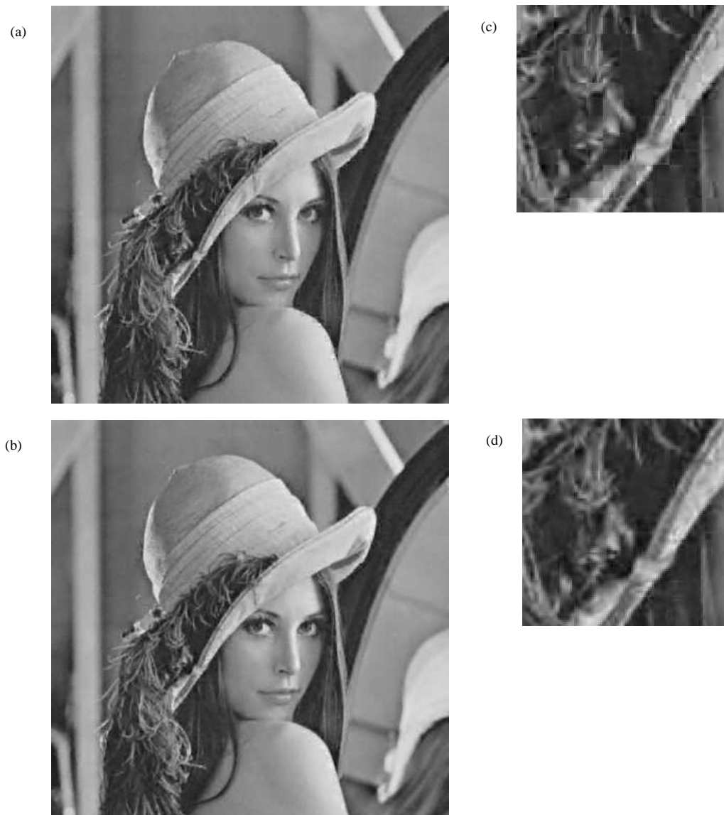
Figure 4.48: Quality comparison of the ‘lena’ image using the GMM-based block quantiser with and without the wavelet transform pre-processing at 0.5 bits/pixel: (a) Without wavelet transform pre-processing (PSNR=31.86 dB); (b) with wavelet transform pre-processing (PSNR=32.62 dB); (c) zoomed up region of image in (a), showing block artifacts; (d) zoomed up region of image in (b)
