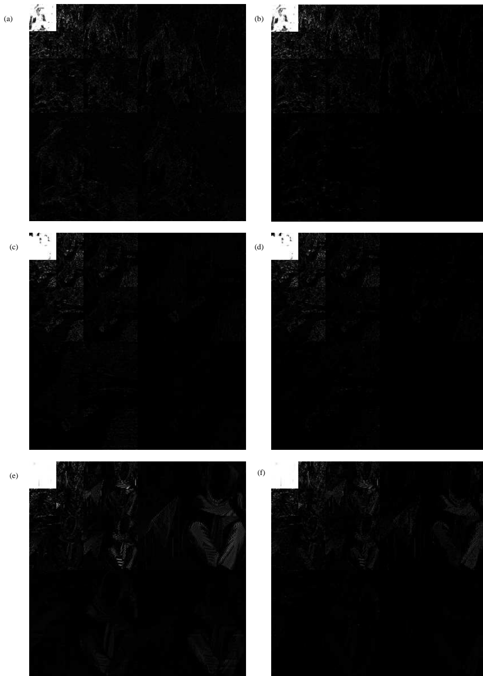
Figure 4.51: Comparing the wavelet transform with the quantised version at 0.5 bits/pixel, showing the preservation of important spatially-localised detail: (a) Wavelet transform of the image 'man'; (b) quantised wavelet transform of the image 'man'; (c) wavelet transform of the image 'vegas'; (d) quantised wavelet transform of the image 'vegas'; (e) wavelet transform of the image 'barbara'; (f) quantised wavelet transform of the image 'barbara'.
