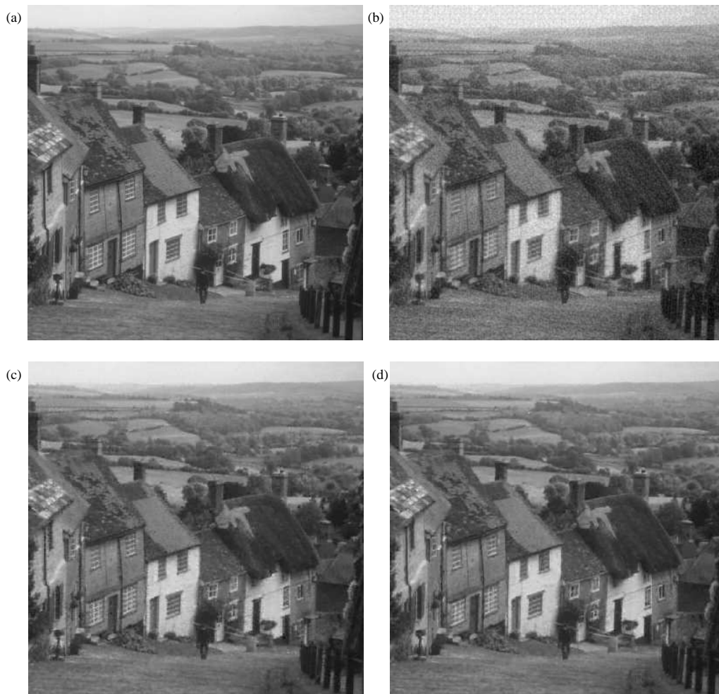
Figure 4.45: Results of the ‘goldhill’ image (part of training set) using the GMM-DCT-based block quantiser with varying number of clusters at 0.5 bits/pixel: (a) original 8-bit image; (b) 1 cluster (PSNR=27.78 dB); (c) 4 clusters (PSNR=29.68 dB); (d) 16 clusters (PSNR=30.40 dB)
