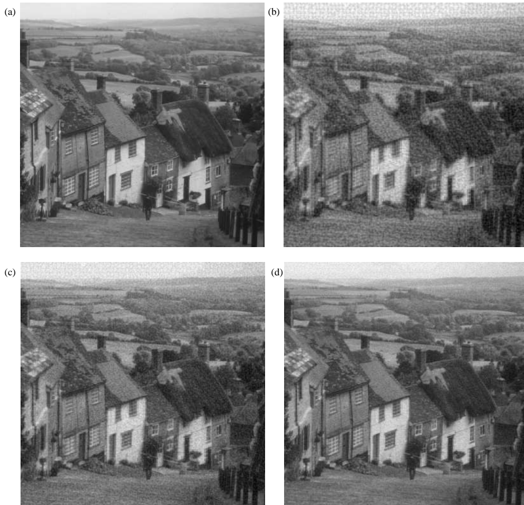
Figure 4.35: Results of the 'goldhill' image at various bitrates (part of training set) using the KLT-based block quantiser: (a) original 8-bit image; (b) 0.25 bits/pixel (PSNR=26.17 dB); (c) 0.5 bits/pixel (PSNR=28.08 dB); (d) 1.0 bits/pixel (PSNR=30.54 dB)
