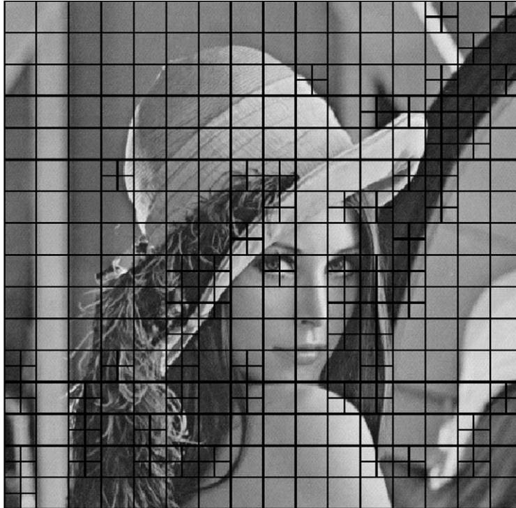
Fig. 2. Quadtree generated using Method 1A and superimposed onto the Lena image.
