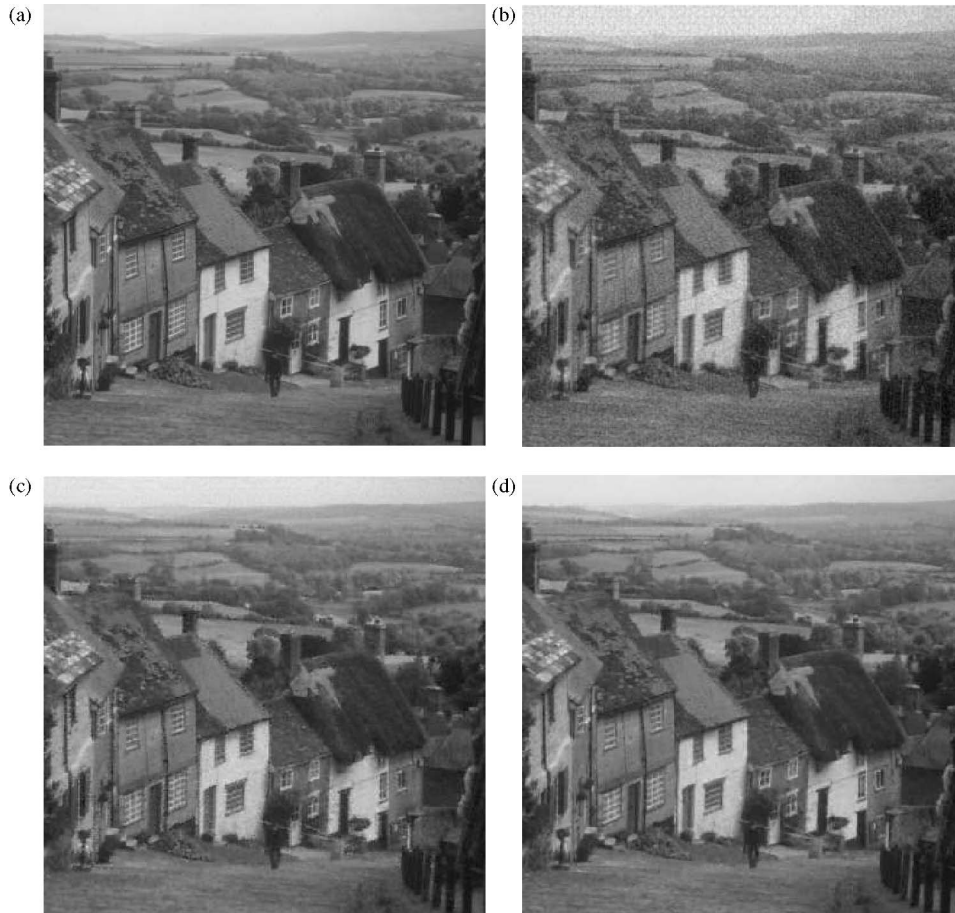
Fig. 4. 'Goldhill' image (part of training set): (a) original 8-bit image; (b) Gaussian KLT-based block quantiser at 0.5 bits/pixel (28.07 dB); (c) GMM-based block quantiser using 2 clusters at 0.5 bits/pixel (29.58 dB); (d) GMM-based block quantiser using 16 clusters at 0.5 bits/pixel (30.74 dB).
