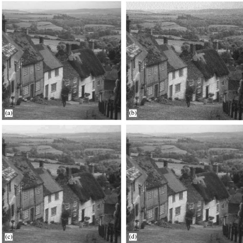
Fig. 7. ‘Goldhill’ image (part of training set): (a) original 8-bit image; (b) single Gaussian DCT at 0.5 bpp (28.69 dB); (c) GMM–DCT with 2 clusters at 0.5 bpp (29.48 dB); (d) GMM–DCT with 16 clusters at 0.5 bpp (30.40 dB).
