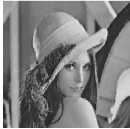
Fig. 9. DCT + Multistage Vector Quantisation (26.42 dB at 0.125 bpp)
