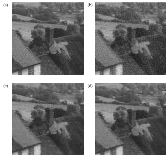
Fig. 8. Part of the image 'goldhill' ( 512 \times 512 ) (a) Original Image (b) Compressed at 0.5 bpp using traditional block quantiser (PSNR 28.16 dB) (c) Compressed at 0.5 bpp using 2 clusters (PSNR 29.48 dB) (d) Compressed at 0.5 bpp using 8 clusters (PSNR 30.15 dB)
